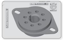
This Cobalt screen capture from THD Electronics, shows a phenolic octal relay socket that is essentially a copy of the old Amphenol tube socket from the '50s.
