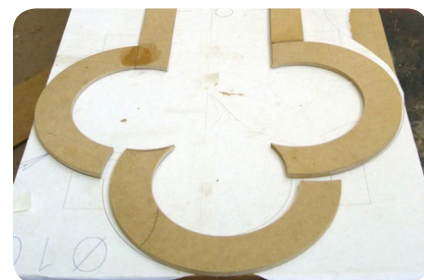
Templates drawn in Xenon are cut out, attached to the wood and used for cutting complex pieces like those of the cross for St. Mary's Cathedral of Austin.
