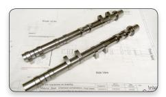
Roberts produces these 260HP inlet cam shafts, that are ground and super finished to specification.
