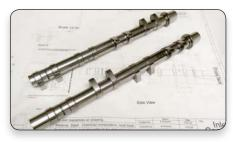
Roberts produces these 260HP inlet cam shafts, that are ground and super finished to specification.
