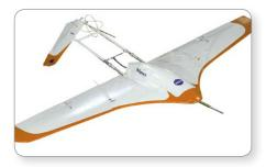
The Kitty Hawk III, created in Graphite, was the first Mars Flyer design to be tested and built. It set an altitude record for unpowered flight. A new, powered version is now in design using Cobalt.
