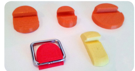
Arnold modeled the ski piercing in Cobalt and printed it in 3D (above). Deciding upon the design, he brought the geometry into Graphite for production drawings (below).
