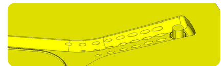
The racquet's injection-moulded thermoplastic includes a textured handle and snap together structure.
