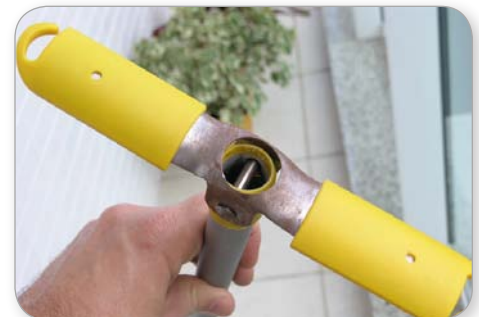
The over-injected handles easily screw the tip into the sand, then flip vertically to receive the upper shaft.
