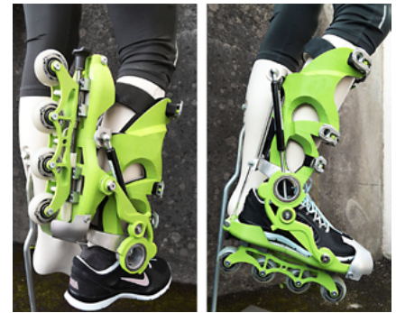
The PowerSwat in closed position, for easy walking and in open position, ready to glide.
