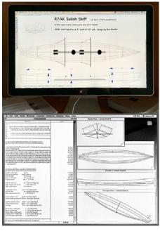
Using specialty hull design software, Mueller then exported a DXF file and brought it into Graphite to designate equipment placement and layout buildable lengths, nested together on 4'x8' sheets of plywood to be cut by his CNC machine.
