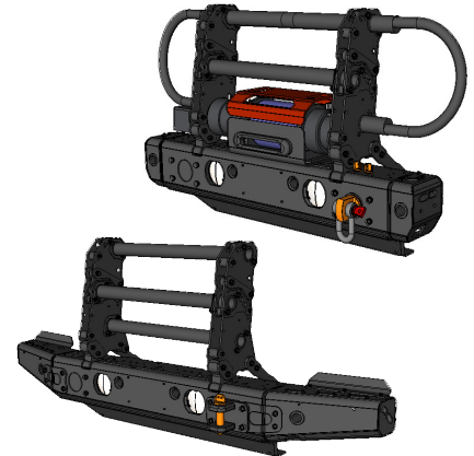
Two of 18 configurations of Pronghorn's Modular Front End System rendered in Cobalt CAD and 3D modeling software.
