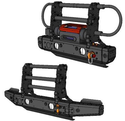
Two of 18 configurations of Pronghorn's Modular Front End System rendered in Cobalt CAD and 3D modelling software.
