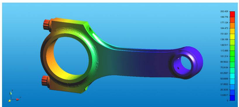
This connector rod was modelled in Cobalt (top) and brought into Iridium for meshing and analysis. The visualizations in Iridium show (middle) the von Mises stress analysis, and (bottom) the displacement.
