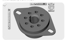
This Cobalt screen capture from THD Electronics, shows a 3D model of a phenolic octal relay socket that is essentially a copy of the old Amphenol tube socket from the 50s.
